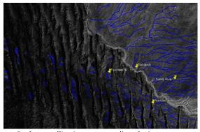
Radar satellite image revealing drainage system
